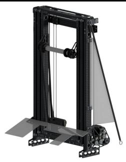
The elevator employs a cascade lift system, ensuring maximum extension speed as all stages move in unison. Constructed from 2" x 1" x 0.0625" aluminum box tubing, the frame remains lightweight yet durable, while the two-stage cascade design enables consistent and reliable access to higher field elements.
