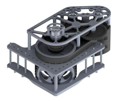
The swerve module provides optimal maneuverability and torque in an all-in-one package. Powered by 2 Kraken motors that control both the angular direction and rotational velocity of the billet wheel. This holonomic drivetrain option ensures a massive advantage for fast and efficient scoring.
