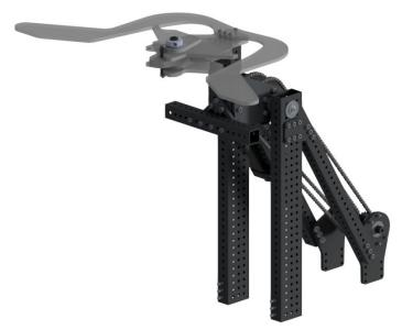
The climber is designed for a secure deep cage grip, allowing the robot to lift its full weight and hold position with minimal backdrive. Constructed from  $2" \times 1" \times 0.125"$  aluminum box tubing, reinforced with  $1" \times 1" \times 0.0625"$  truss supports, it maintains high rigidity and strength, ensuring a stable and reliable climb every match.
