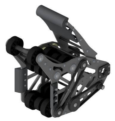
The end effector system is built to quickly and consistently intake and score both coral and algae. Several sets of rollers quickly intake and align the coral so that scoring is fast and consistent. Both the coral and algae systems are driven by a single Kraken X60 motor.
