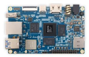
The vision pipeline runs separately from the robot code on each coprocessor, and sends positional data to the robot code. The code then factors the tag detections from the cameras into a Kalman filter along with the encoder odometry from the swerve drive to get an accurate reading of the robot's position. The filter also weighs sensor results using results from our empirical tests to negotiate the best position and discard bad data.
