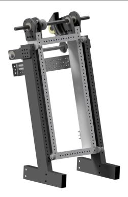
The elevator utilizes a cascade lift to provide maximum speed in extension, since every element moves in unison. A curved guard helps to protect the pivot from damage. The elevator has a strong frame to support the whole shooter subsystem while being lightweight to increase speed and the amount of power needed to move.
