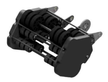
The shooter pivots on an axle connected to the elevator, allowing it to position for a variety of shots. Six sets of rolling compliant wheels swiftly launch the note from the shooter.
