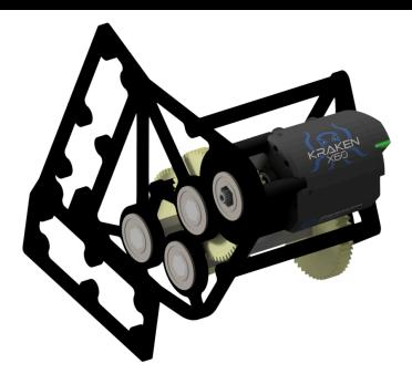
This custom gearbox system utilizes a Kraken X60 motor driving a set of gears to smoothly extend the elevator as it translates, and give the elevator enough power to lift the robot and prevent significant backdrive.
