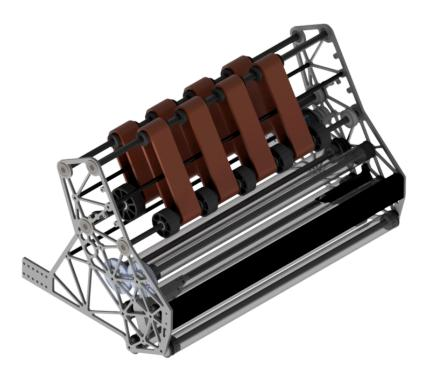
The intake pulls in notes as soon as it touches them, allowing for faster cycle times and a quick pickup for drivers. Notes rapidly move through a series of rollers, belts, and wheels to position correctly in the shooter for an accurate shot. The intake must work every time, as one failure, break, or jam prevents the robot from being offensive for the majority of the match.
