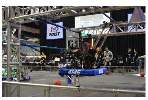
The WorBots are at the high school level of the *FIRST* program, meaning we build robots that are approximately 120 pounds. For the first fifteen seconds, the robot runs off of programming alone, and then it is controlled by the driver for the remaining time.
